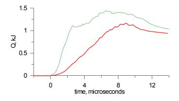
Fig.(4.4)3. Dynamics of the full plasma energy content by diamagnetic measurements. The standard operating mode is shown by the thin line, the mode with smooth increase in energy of electrons by the thick line.
