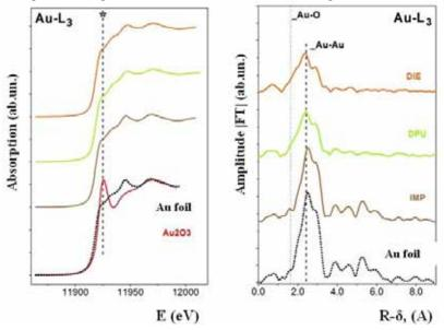
Fig.(6.1)30. XANES spectra (Au- $L_3$  edge; \* indicates the white line) and atomic radial distribution (ARD) functions of the local environment of gold for these samples and frames of reference.
