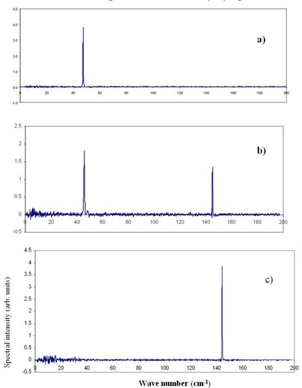
Fig.(6.3)1. Laser generation of the terahertz FEL at the first (a), first and third (b), and third (c) harmonics.
