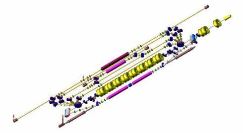
Fig.(6.3)21. Scheme of the full-scale 4-track accelerator-recuperator (plus one track in the vertical plane with the FEL for the THz range of 110-240 microns).
