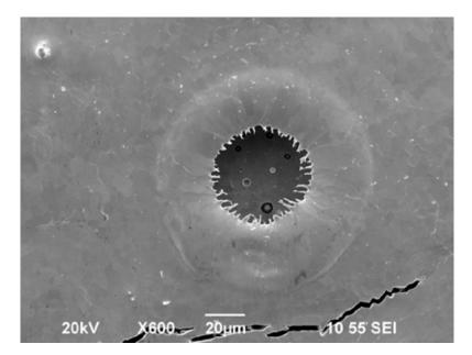
Fig.(4.4)9. Even moderate energy loads (5 pulses with energy density 2 MJ/m<sup>2</sup> per shot) leads to tungsten surface strong melting and formation of deep bubbles and cracks.
