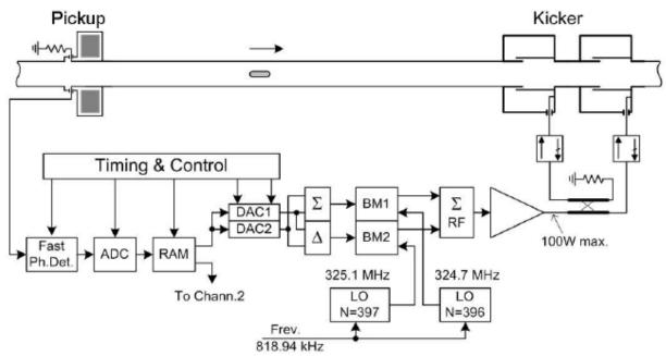
Fig.(5.2)8. Block diagram of the VEPP-4M longitudinal feedback.
