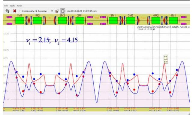
Fig.(5.1) 9. Beam sizes and envelopes.
