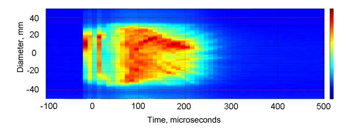
Fig.(4.4)15. Dynamics of plasma brightness (slit scan). Preliminary plasma starts at  $-35 \mu$ s, the beam starts at 0  $\mu$ s.
