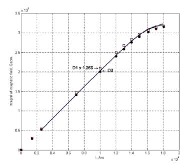
Fig.(2.1)2. Field integrals of magnets D1 and D3 along the electron beam trajectory in dependence on the current of the coils of the magnets. The black dots show the results of measurements of magnet D1 (multiplied by a "correct" coefficient of 1.266); the hollow squares are for the measurements of magnet D3. The solid and dashed lines present the results of the calculation of magnets D1 and D3 by the MERMAID program.
