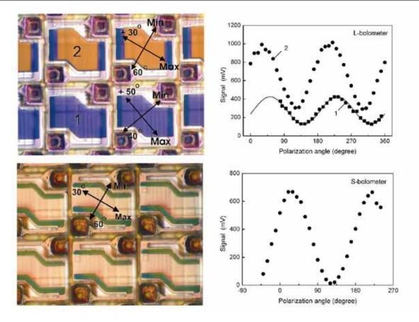
Fig.(6.3)10. Dependence of the sensitivity of microbolometer arrays of different types depending on the direction of terahertz radiation polarization. The sensitivity increases when a thin metal layer is applied to the surface of the sensor of the L bolometer (top graph).
