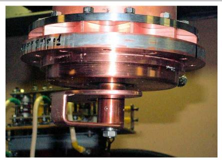
Fig.(7.5)5. Coupling loop of the power input.
