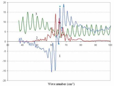
Fig.(6.3)2. Fourier spectra of rotation angles (1, degrees), circular dichroism (2, dichroism intensity  $\times$  50), and transmission (3, transmission  $\times$  30) and data of measurement on the FEL (dots) for a square grid of microcoils on a 400 µm GaAs substrate. The FEL line width is 0.2 cm<sup>-1</sup>.
