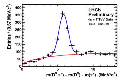
Fig.(1.9)2. Signal D\* $\rightarrow$ D $\pi$ , D $\rightarrow$  K<sub>s</sub> $\pi\pi$  observed by the LHCb detector with a statistics of 124 nb<sup>-1</sup>.
