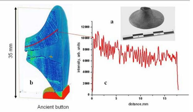
Fig.(6.1)27. Examination of a wooden article by the method of computer X-ray tomography: (a) general view of a quiver plate, (b) cross-section of the object with the radius of measurement, (c) density curve, reflecting the variability of the width of tree rings.
