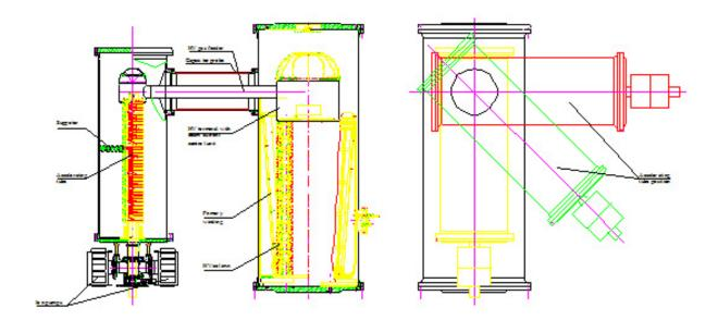
Fig.(8.1)3. Variant of assembly of accelerator with remote accelerator tube
