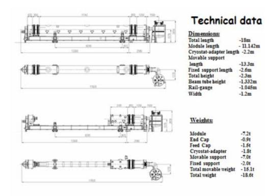
Fig.(5.10)5. Technical specifications of the BINP equipment.
