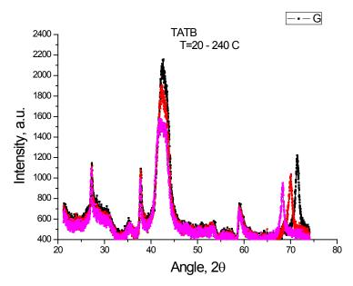
Fig.(6.1)6. Dynamics of the positions of diffraction peaks in TATB heated from 20° to 240° C.
