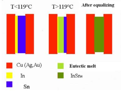
Fig.(6.1)21. Scheme of the contact thermosetting soldering using the In-Sn system.
