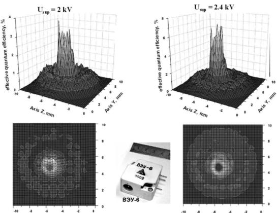
Fig.(6.2)2. Band characteristics of SEM-6 at a photon energy of 268 eV and dynode supply voltages of 2kV and 2.4 kV.
