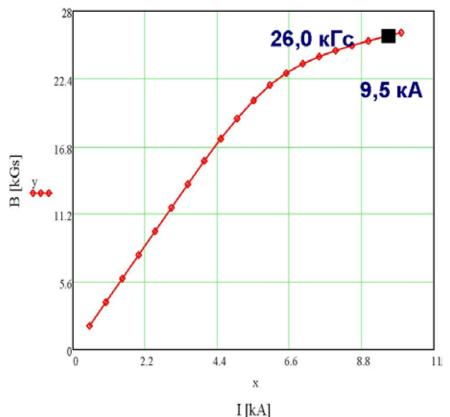
Fig.(5.1)13. Calculated saturation curve of BEP magnetic field in gap of 32 mm.
