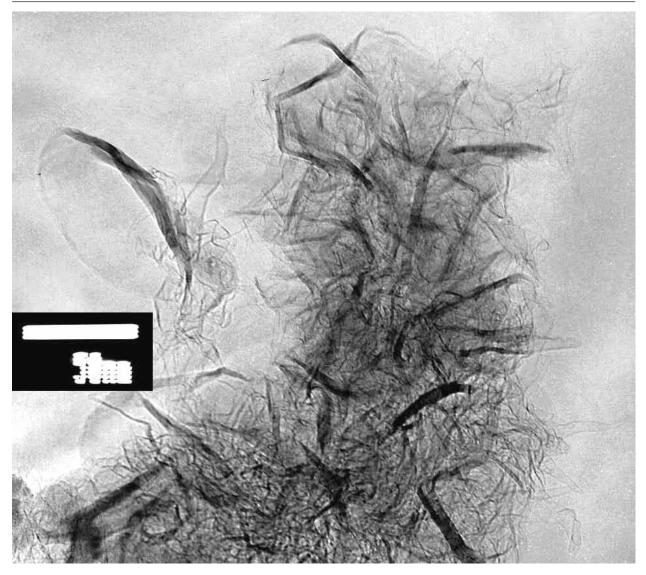
Fig.(8.1)7. Accumulation of nanohornes
