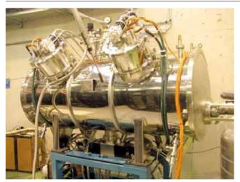
Fig.(6.4)1. Testing the 119-pole wiggler with a field of 2.2 T and a period of 31 mm on the ALBA-CELLS (Spain) storage ring.
