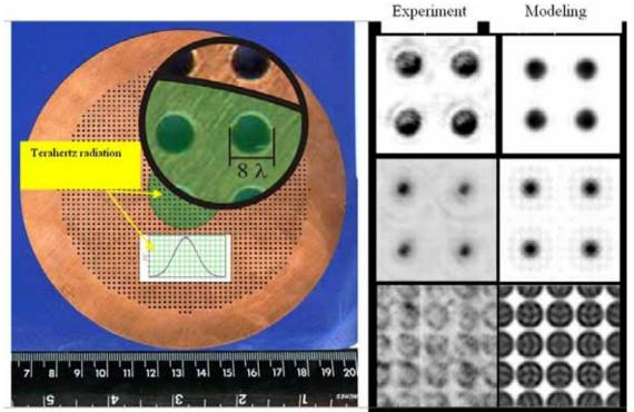
Fig.(6.3)11. Left: one of the periodic structures used to study the Talbot effect in the terahertz range. Right: comparison of numerical simulation and images recorded from some characteristic planes using a microbolometer array.
