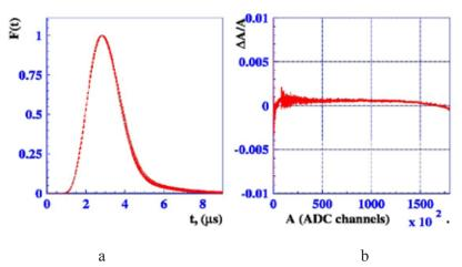
Fig.(1.10)9. (a) Pulse shape after the shaper; (b) Deviation from the linear dependency of the shaper module.
