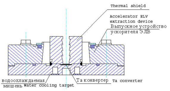
Fig.(8.1)2. Cross-section of bremsstrahlung converter
