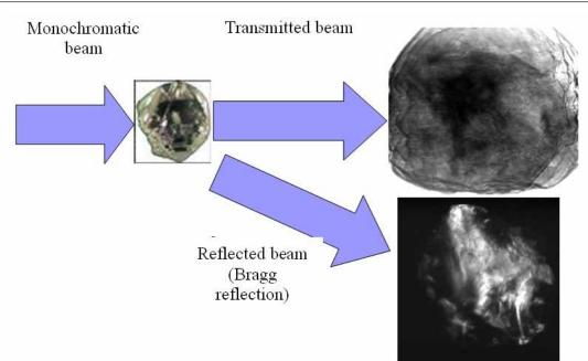
Fig.(6.1)22. Images of diamond in the passed beam and in radiation reflected at the Bragg angle.
