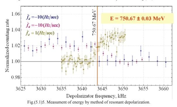
As one can see from Fig.(5.1)5 a jump of the counting rate occurs in narrow region of depolarizer frequencies, so we can determine beam energy as  $E=750.67 \pm 0.03$  MeV. The energy value obtained is in good agreement with expected one, which is based on magnetic measurements and energy calibration by mass of  $\varphi$ -meson resonance.
