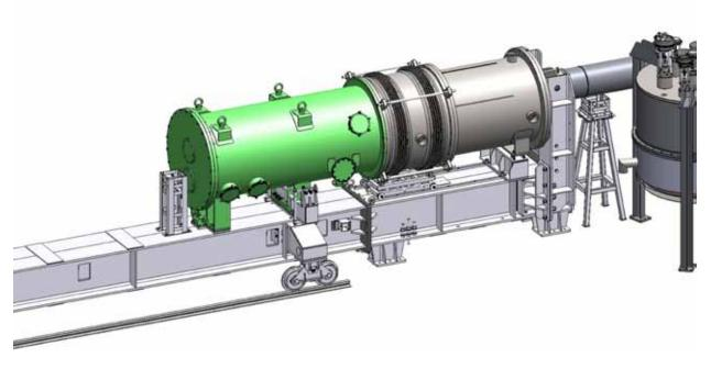
Fig.(5.10)9. Testing an individual resonator with a cryostat adapter.
