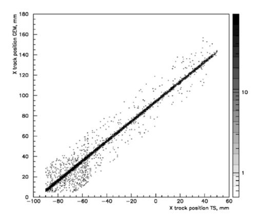
Fig.(1.8)5. Correlation of track coordinates recorded in a hodoscope on drift tubes (horizontal axis) and in a GEM SRSE detector (vertical axis).
