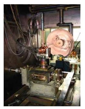
Fig.(7.13)3. Drift tube in the chamber of the EBW device.
