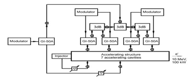
Fig.(8.2)4. ILU-14 block diagram.
