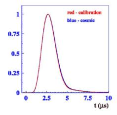
Fig.(1.10)11. Shapes of the signal from the CsI(Tl) counter (blue) and the signal of the calibration module (red).
