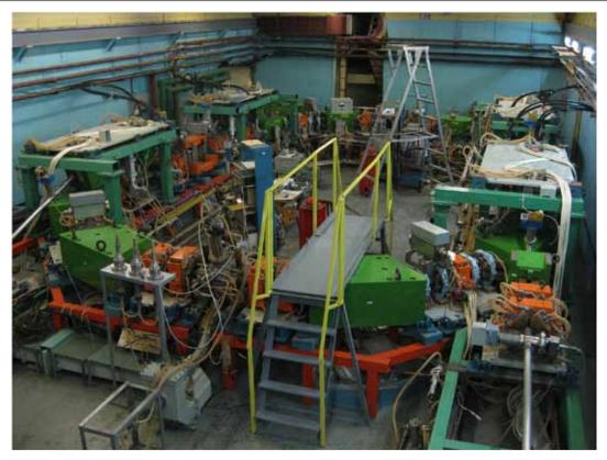
Fig. (5.3)4. The system of positron inlet-outlet for storage ring is prepared for operation.
