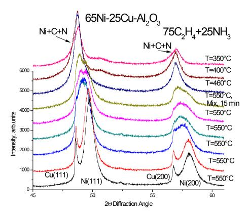
Fig.(6.1)14. Phase transformations of the nickel-copper catalyst for CNF synthesis in the course of reaction at different temperatures.
