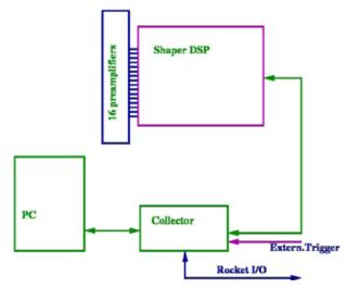
Fig.(1.10)10. Scheme of the calorimeter modules operation in stand-alone mode.
