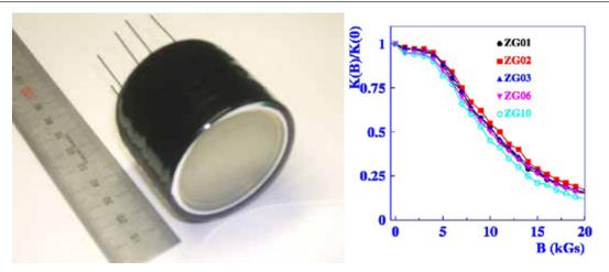
Fig.(1.10)12. Vacuum photopentrode by Hamamatsu company.
