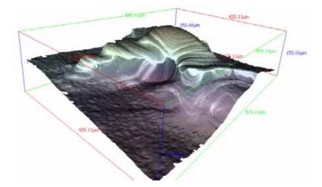
Fig.(4.4)13. 3D view of tungsten surface after 9 GOL-3 pulses with energy density 4  $MJ/m^2$  per shot. Hills height is more than hundred  $\mu m$ .
