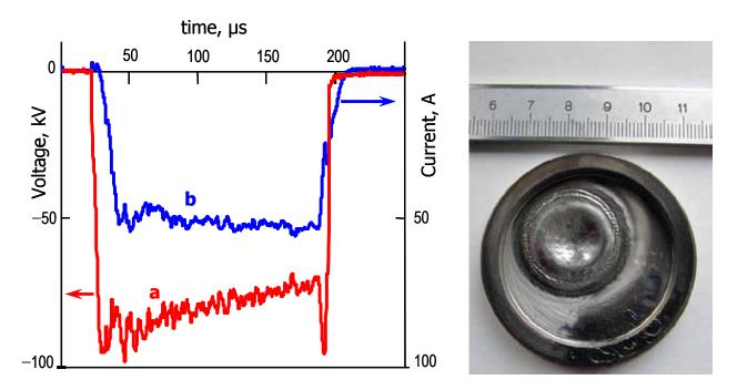
Fig.(4.4)16. Typical waveforms of the beam and imprint on the end cap of the drift tube (50 cm from the EOS).
