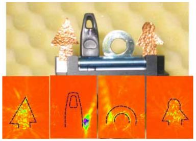
Fig.(6.3)12. Images of objects in the terahertz region, taken with the Fresnel lens and a microbolometer array.
