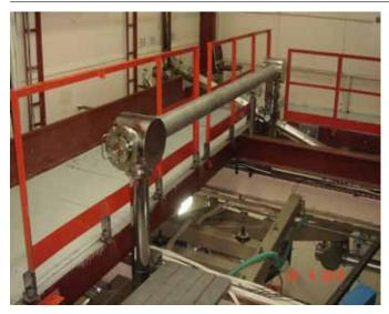
Fig.(6.3)22. Radiation extraction beamline of the second stage FEL (middle part). Radiation coming from below is reflected from two mirrors and gets into the "old" part of the beamline (in a distance) through the movable mirror assembly.
