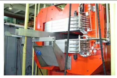
Fig.(6.4)2. Radiation-resistant dipole magnet at the bench for magnetic measurements.
