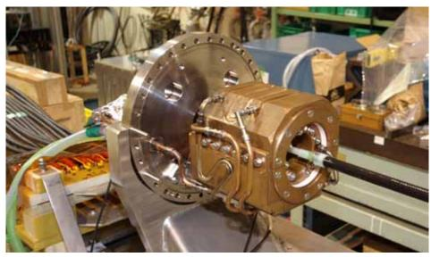
Fig.(5.13)2. Pulsed magnet for the positron source of the KEK Super-B Factory.
