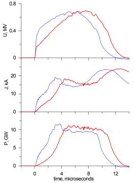
Fig.(4.4)2. Main parameters of the electron beam for two cases: the standard mode (thin lines) and the mode with smoothly increasing cathode voltage (thick lines). Typical waveforms of the diode voltage (top), the beam current (middle) and the beam power (bottom) are shown.
