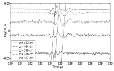
Fig.(4.4)8. Longitudinal correlation of the bursts. Zero lines are shifted proportionally to the coordinates of probes (from bottom to top: 167, 288, 398, 464, and 492 cm), slope of dotted lines corresponds to the mean Alfven velocity.
