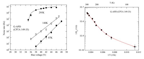
Fig.(1.8)1. Characteristics of the "CPTA 149-35" G-APD at cryogenic temperatures. Left: rate of singleelectron noise in dependence on bias voltage. Right: dependence of quenching resistance pixel on temperature.
