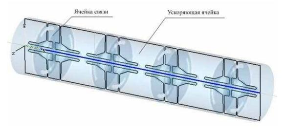
Fig.(8.2)2. Accelerating structure of the prototype.
