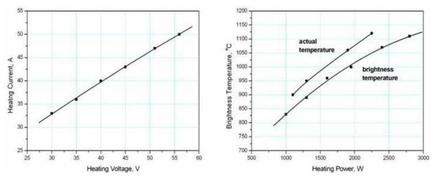
Fig. (5.6)5. Heating and temperature characteristics of the cathode of LIA – 2.
