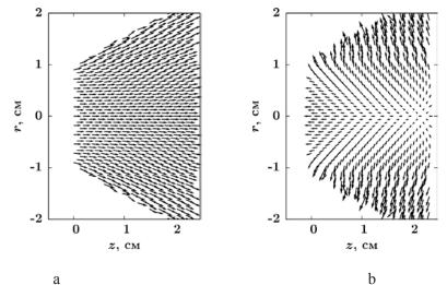
Fig.(6.1)2. The velocity field in the system associated with the detonation wave front (a) and in a fixed system (b) behind the TATB detonation front.
