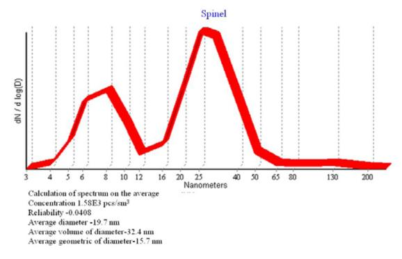
Fig.(6.3)8. Fractional composition of spinel from data of non-invasive ablation.
