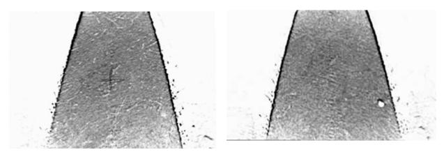
Fig.(6.1)5. Plasticized TATB. Room temperature (left). A temperature of 200° C (right). A 60 µm cavity can be seen.
