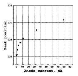
Fig.(1.10)13. Dependency of the <sup>137</sup>Cs peak position on the average anode current of the photopentrode.
