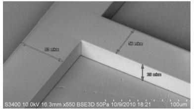
Fig.(6.1)7. Fragment of a work-piece for X-ray mask – a microstructure of the SU-8 resist 29  $\mu$ m high on a glassy-carbon substrate.
