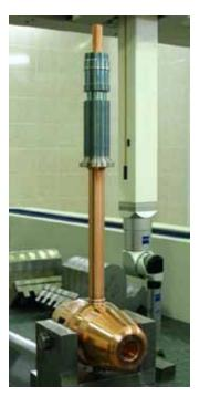
Fig.(7.13)2. Pilot sample of the drift tube.
