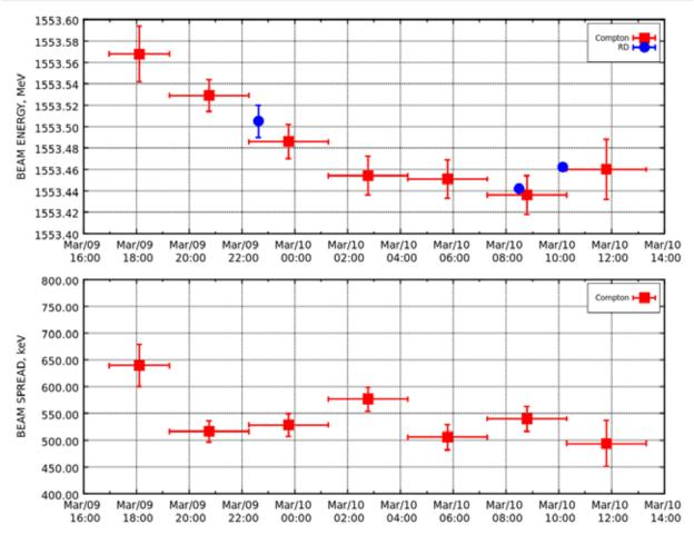
Fig.(5.2)4. Measurement of the VEPP-4M beam energy by the CBS and RD methods.
