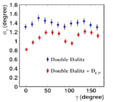
Fig.(1.9)6. The accuracy of measuring the angle  $\gamma$  in dependence on its value for the method of «double Dalitz analysis" for a statistics content of 50 fb<sup>-1</sup> (after upgrading the LHC and LHCb).
