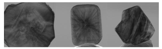
Fig.(6.1)23. Topographs of diamonds with different morphology, made in transmitted radiation.
