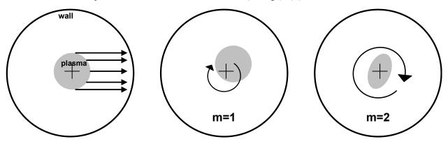
Fig.(4.1)2. Simplified scheme of plasma column motion without vortex confinement (left) and with vortex confinement realization (center and right): according to theoretical model only m = 1 and m = 2 modes are available at differential rotation.
