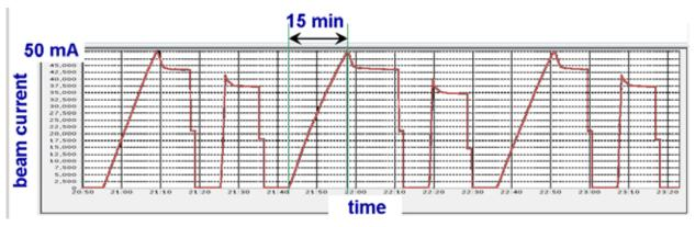
Fig.(5.2)6. VEPP-3 beam current as a function of time.
