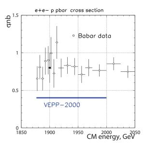
Fig.(1.2)1 Cross section of the  $e^+e^- \rightarrow p\bar{p}$  process. the black dot shows the preliminary result of the SND measurement using a part of the accumulated experimental data. For comparison, results of the previous measurements of BaBar is also shown.
