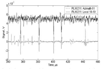
Fig.(4.4)7. Correlation of pulsed magnetic activity and neutron/gamma emission. Above: local neutron/ gamma radiation detector data; below: azimuthal magnetic probe data.
