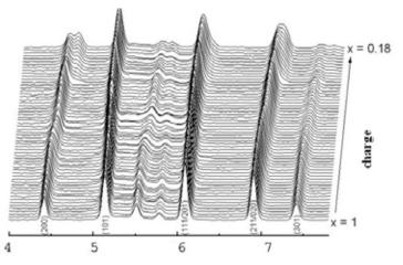
Fig.(6.1)19. Diffraction patterns obtained in the course of charging LICs.
