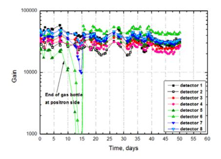
Fig.(1.8)3. Coefficient of gas amplification of the GEM SRSE detectors in dependence on time.
