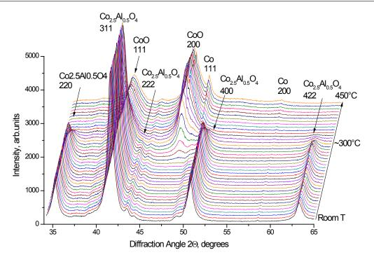
Fig.(6.1)15. The process of cobalt reduction from the solid solution of  $Co_{2,5}Al_{0,5}O_{4}$  in a hydrogen flow.
