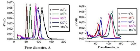
Fig.(6.1)12. Shows the distributions of pore volumes on sizes for silicon oxide and alumina-silicate material, calculated from nitrogen adsorption isotherms at 77 K which were measured on the automated adsorption unit ASAP - 2400 (Micromeritics). With increasing temperature of hydrothermal treatment the size of material pore also increases due to the surfactant thermal expansion prior to polycondensation of the silicate wall.
