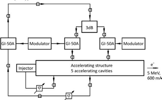
Fig.(8.2)1. Accelerator prototype block diagram.
