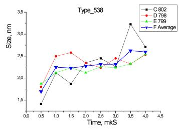
Fig.(6.1)4. Evolution of the growth of nanoparticle size over time at TATB detonation. The mean particle size is shown in curve F.
