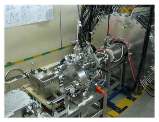
Fig. (5.4)2. Accelerator target assembly and front part of accelerator.
