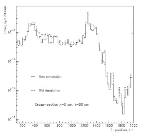
Fig.(1.9)1. Dependence of the absorbed dose on the z coordinate.
