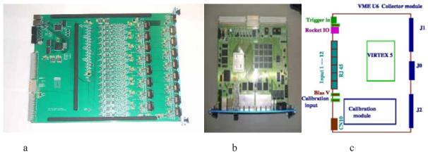
Fig.(1.10)8. (a) 16-channel shaper-digitizer electronic module in the VME standard; (b), (c) Concentrator electronic module in the VME standard.
