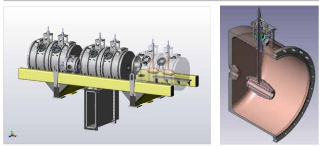
Fig.(7.13)1. Left: the CCDTL accelerating module. Right: half of the CCDTL accelerating cavity with the drift tube inside (cross section).
