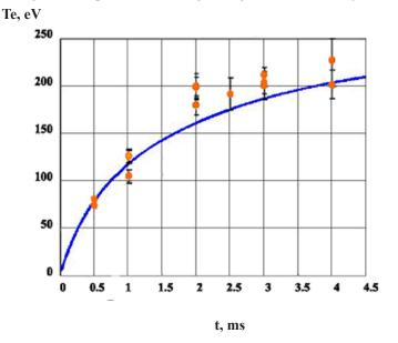
Fig.(4.1)6. Electron temperature vs time in the regime with injection of 4.8 MW deuterium beams into deuterium plasma: points - result of measurement, the line - result of "zero-dimensional" model taking into account the longitudinal losses in the gas-dynamic regime.
