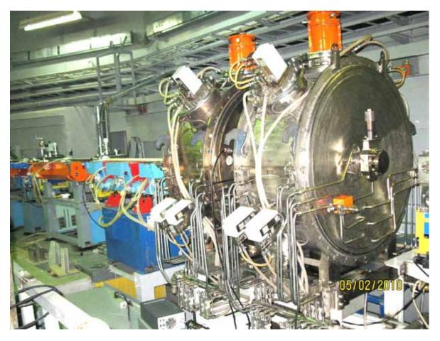
Fig.(7.9)1. Two accelerating cavities in the 2.2 GeV storage ring.
