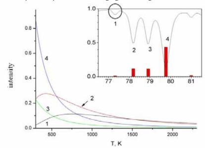
Fig.(6.3)13. Change in the relative intensity of four water-vapor absorption lines in the interval of 77 - 80 cm<sup>-1</sup>. The inset shows the corresponding portion of the spectrum of water vapor at room temperature. The circle indicates the line chosen for the measurement.
