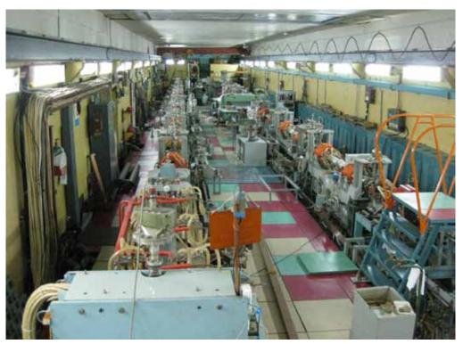
Fig.(5.3)1. Linear positron accelerator of VEPP – 5 IC.
