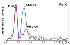
Fig.(6.1)33. Curves of atomic radial distribution in the local environment of palladium for the samples of ~ 0.2 Pd-20%Ce-ZrO<sub>x</sub>/Al<sub>2</sub>O<sub>3</sub> and ~ 1% Pd/Al<sub>2</sub>O<sub>3</sub> (frame of reference).
