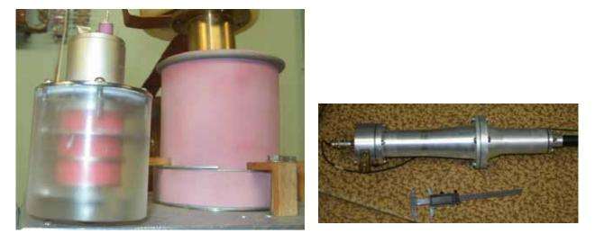
Fig.(5.14)1. Thyratrons TPI1-1k/35 and TGI1000/25 and a 50 ohm load (from left to right).
