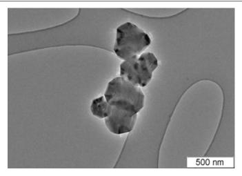
Fig. (6.3)5. Electron microscopy of particles produced by the powerful effect of FEL radiation on graphite.
