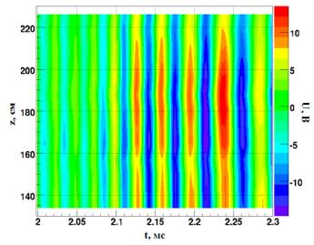
Fig.(4.1)5. The signal from the Mirnov probe depending on the longitudinal coordinate z and time t.
