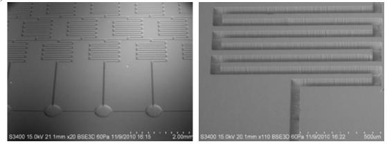
Fig.(6.1)9. SEM photos of fragments of the microchannel module.
