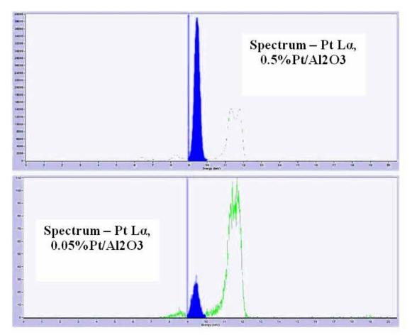
Fig.(6.1)34. Energy spectrum for the samples of ~0.5%Pt/Al<sub>2</sub>O<sub>3</sub> and ~0.05%Pt/Al<sub>2</sub>O<sub>3</sub>.
