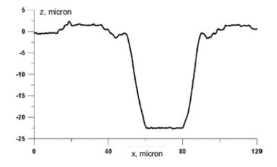
Fig.(4.4)10. Depth profile of bubble on tungsten surface. Measured by MeX software by using of SEM stereopair.
