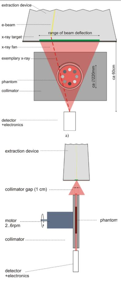
Fig.(8.1)1. Longitudinal (a) and cross-section (b) view of simulation computed tomography installation
