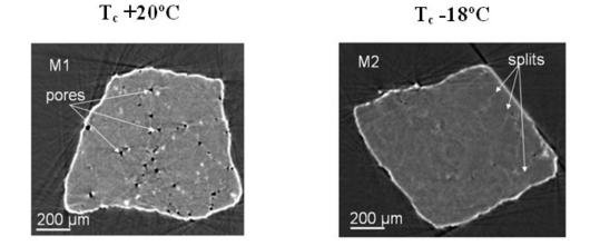
Fig.(6.1)26. EM samples based on the FTDO/DNP mixture, obtained at various temperatures of crystallization.
