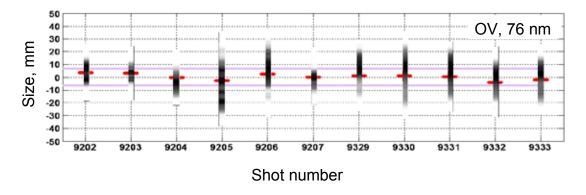
Fig.(4.4)14. Size and position of VUV-emitting plasma in a sequence of shots with the beam injection into a non-ionized deuterium. Shades of gray shows brightness and position of the plasma, its center is marked by a thick dash, expected beam diameter is shown as horizontal solid lines.
