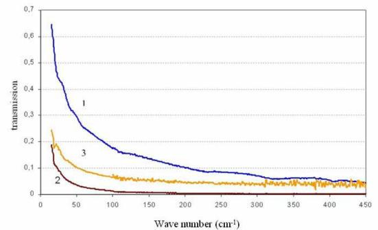
Fig.(6.3)3. The transmission spectra of samples of nanotubes for radiation polarized normally to the nanotube axes (1, upper curve) and along the nanotube (2, lower curve) and their ratios (3).
