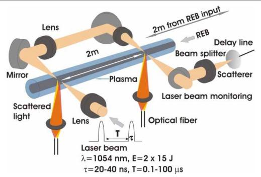
Fig.(4.4)4. The layout of upgraded Thomson scattering system for measurement at two spatial points and at two time instants within a single plasma discharge.
