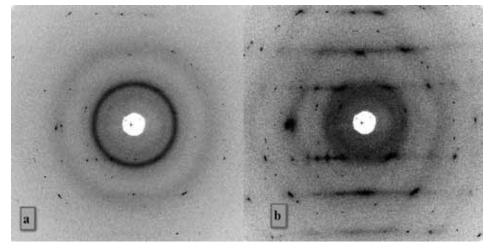
Fig.(6.1)20. Fragments of diffraction patterns obtained in the course of eutectic crystallization: (a) 5 minutes after the onset of crystallization; (b) 12 minutes after the onset of crystallization.
