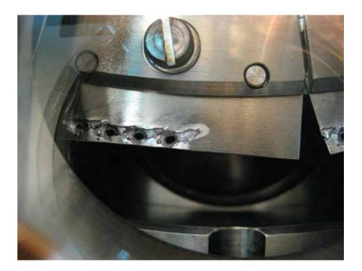
Fig. (5.4)5. Target of LIA – 2 with holes burned up by an electron beam.
