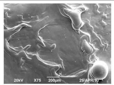
Fig.(4.4)12. SEM image of tungsten surface after 9 GOL-3 pulses with energy density 4 MJ/m<sup>2</sup> per shot corresponding to biggest ELM type I in ITER divertor (expected 10<sup>3</sup> ELM per ITER shot).
