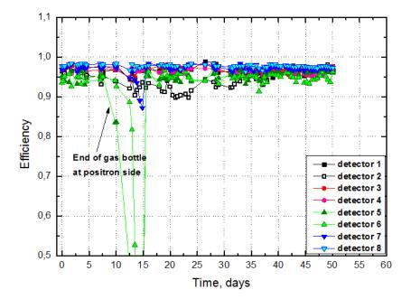
Fig.(1.8)4. Effectiveness of the GEM SRSE detectors in dependence on time.
