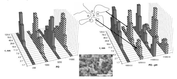
Fig.(6.3)9. The size distribution of particles produced by ablation of PVA samples of different polymerization degrees (PD) and composite particles formed at an equimolar ratio PVA/silicic acid and different pH values. A microphotography of the composite precipitate in the PVA - silicic acid system at an equimolar ratio of the components and pH = 10, a scale of 1  $\mu$ m, and a schematic structure of the composite nanoparticles.
