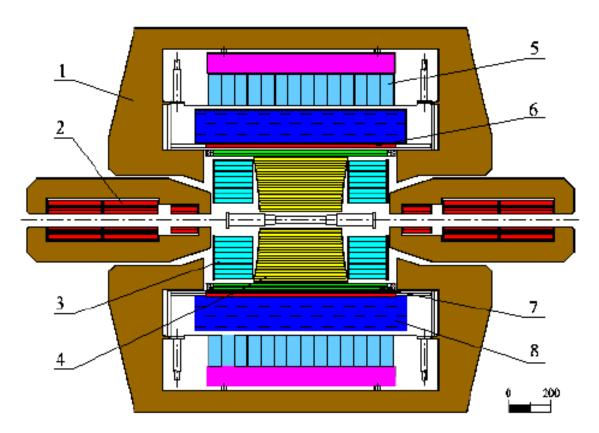
Fig.(1.1)1. CMD-3 detector. 1 – the magnet yoke, 2 – the superconducting solenoids of VEPP-2000, 3 – the crystal-BGO electromagnetic calorimeter; 4 – the drift chamber; 5 – the crystal-CsI electromagnetic calorimeter; 6 – the superconducting solenoid of CMD-3, 7 – the Z-chamber, 8 – the liquid-xenon electromagnetic calorimeter.
