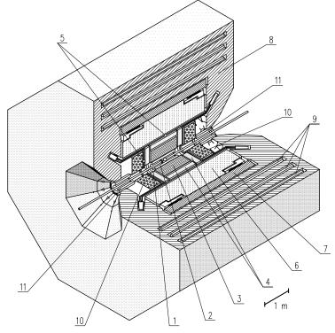
Fig.(1.3)1. The KEDR detector. 1 - vacuum chamber of the collider, 2 - vertex detector, 3 - drift chamber, 4 - aerogel Cherenkov counters, 5 - time of flight counters, 6 - liquid krypton barrel electromagnetic calorimeter, 7 - superconducting solenoid, 8 - magnet yoke, 9 - muon chambers, 10 - end cap electromagnetic calorimeter based on CsI crystals, 11 - compensating solenoid.
