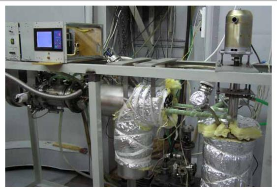
Fig. (5.5)4. Welding gun on the shielding window test stand with liquid lead.
