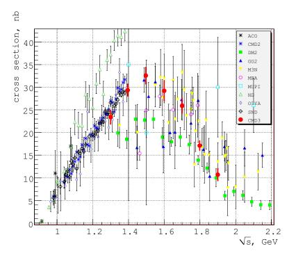
Fig.(1.1)2. Energy dependence of the cross section of production of four charged pions, obtained with the CMD-3 detector on the VEPP-2000 collider, in comparison with results of other experiments.
