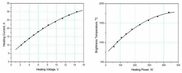
Fig. (5.6)3. Heating and temperature characteristics of the cathode unit ILU - type 20 mm in diameter.
