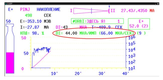
Fig.(5.2)5. Accumulation of positrons in the VEPP-3 booster storage ring.
