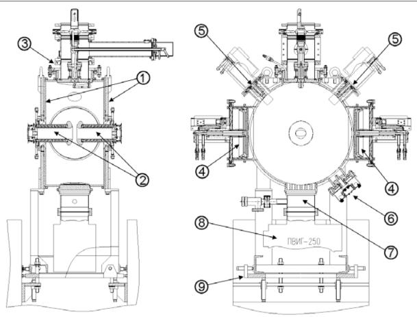
Fig.(5.1)14. New RF cavity for BEP.
