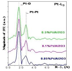
Fig.(6.1)35. Curves of atomic radial distribution in the local environment of platinum for the studied model test platinum samples.
