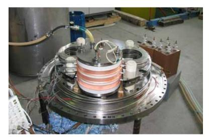
Fig.(5.7)2. Transformer section under testing.
