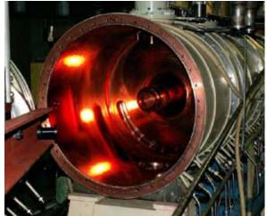
Fig.(7.5)3. View of the accelerating cell during the assembly of the structure.
