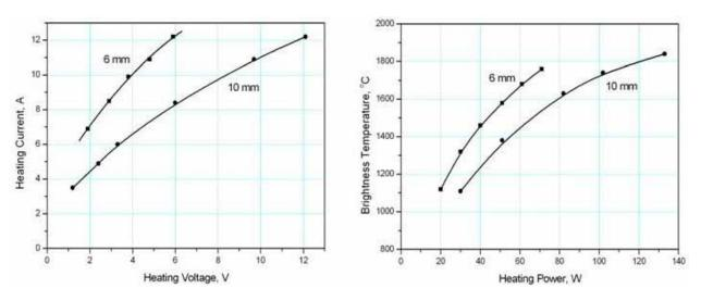
Fig. (5.6)2. Heating and temperature characteristics of the ELV-type cathodes.
