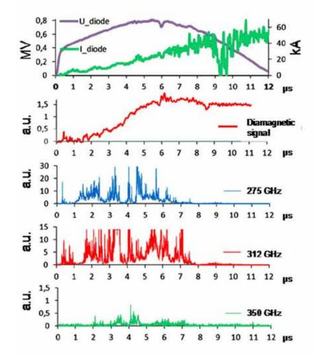
Fig. (4.4)6. Typical waveforms which characterize the stage of collective plasma heating by the relativistic electron beam in GOL-3. Shown from top to bottom are: the cathode voltage of the beam generator and the beam current; diamagnetic plasma pressure at coordinate z = 77 cm; signals of detectors of terahertz radiation located at coordinate z=83 cm. Central wavelengths of the bandpasses of the spectral system are designated for each detector.
