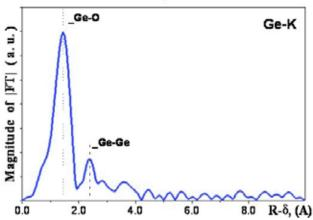
Fig.(6.1)36. Curves of atomic radial distribution in the local environment of germanium for the studied geologic samples (a conglomeration of bacteria and fungi, which accumulate germanium compounds) from geothermal sources (Lake Baykal,~50 ppm of Ge).
