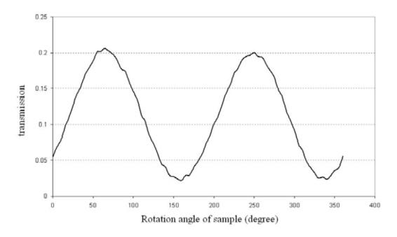
Fig.(6.3)4. Polarization angle characteristic of one of the samples with aligned carbon nanotubes.
