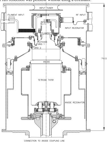
Fig.(7.7)1. Arrangement of a TH781 tetrode in the body of the tube module of the generator.
