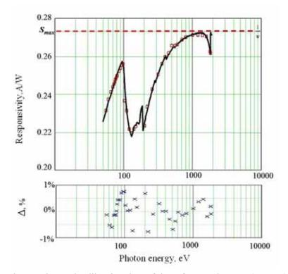
Fig.(6.2)1. Upper graph: experimental calibration data of the reference detector (squares) and approximation of the data (solid line). The horizontal dotted line marks the level of maximum achievable sensitivity for the silicon photodiode (Smax). Lower graph: difference between the calibration data and the function approximation, %. All data are in the error corridor of  $\pm 1\%$ .
