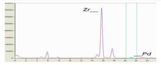
Fig.(6.1)32. Energy spectrum for the nanosysystem of ~ 0.2 Pd – 20% Ce-ZrO<sub>X</sub>/Al<sub>2</sub>O<sub>3</sub>.
