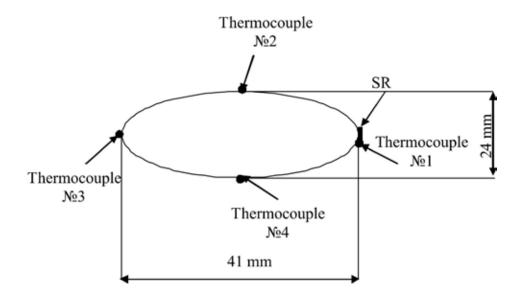
Fig.(5.10)12. Arrangement of thermocouples on the prototype vacuum chamber.
