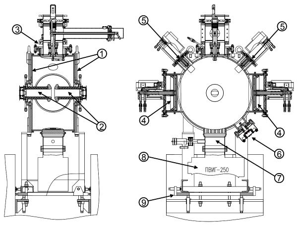
Fig.(7.11)1. The resonator structure: 1 - the bi-metal walls, 2 - the coaxial inserts, 3 - the power input, 4 - the mechanisms for frequency retuning, 5 - the mechanisms for HM retuning, 6 - the measuring loop, 7 - the vacuum pumping port, 8 - the vacuum pump, 9 - the stand.
