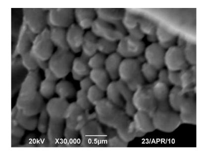
Fig.(4.4)11. Crack pattern with cell sizes 0.3 µm on tungsten surface after irradiations.
