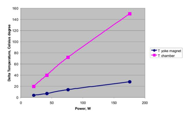
Fig.(5.10)11. Dependence of heating on power.
