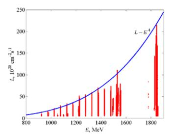
Fig. (5.2)2. Measured and calculated luminosity as a function of beam energy.
