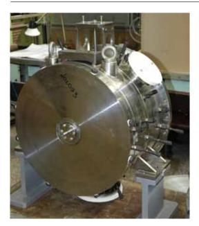
Fig.(7.13)4. The body of the cavity of the 1st module is prepared for vacuum tests.
