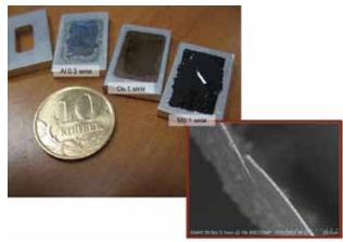
Fig.(6.2)3. General view of the filters and a micrograph of a cleavage of Mo film. The thickness is approximately 1 micron. Work is underway to improve the homogeneity and mechanical strength of the molybdenum filters.
