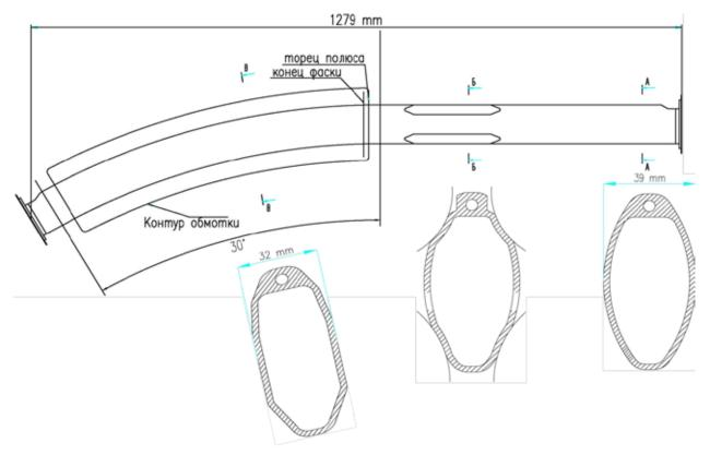
Fig.(5.1)15. Improvements in vacuum chamber of BEP.
