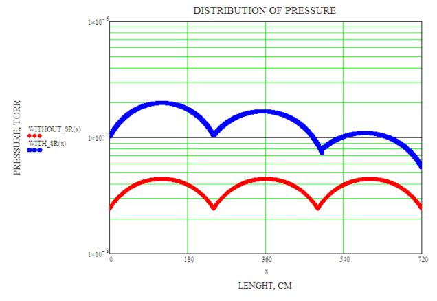
Fig.(5.10)10. Pressure distribution in the straight section.
