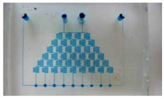
Fig.(6.1)10. Photo of a disposable replaceable microfluidic module – gradientator for positioning cells of genosensors. For clarity, the channels are filled with ink. These measurements showed that microfluidic modules fabricated by the LIGA technology fully correspond to the topology, design documentation, and specification requirements. The width of channels of different modules is 55 microns to 60 microns. The roughness was less than 3%.
