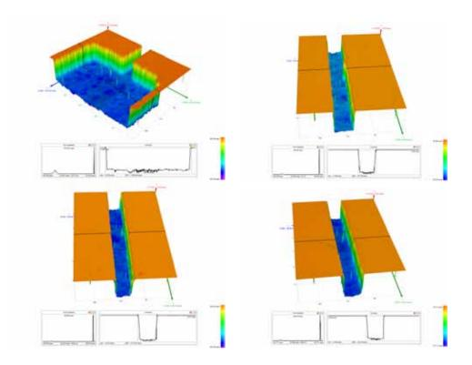
Fig.(6.1)11. Quality control of manufacturing of microfluidic modules using the profilometer Profile (TDI DT SB RAS).
