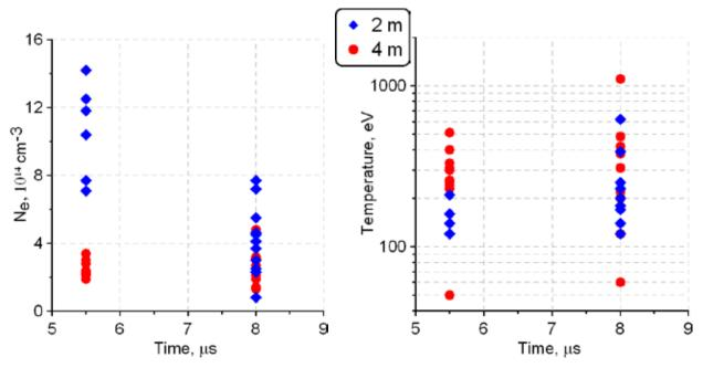
Fig. (4.4)5. Dynamics of density and mean energy of plasma electrons during the plasma heating at distance of 2 m and 4 m from input plug. Data are obtained from Thomson scattering measurements during several plasma discharges.
