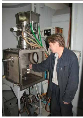
Fig. (5.5)1. The electron – optic column with indirect cathode heating (by electron beam) on the experimental chamber.
