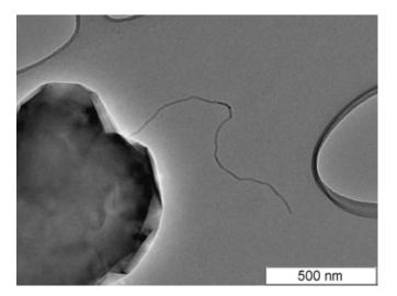
Fig.(6.3)7. The carbon nanotube.
