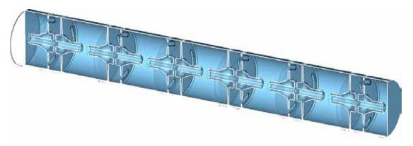
Fig.(8.2)3. ILU-14 accelerating structure.
