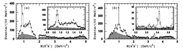
Fig.(1.10)5. Invariant mass distributions of  $K^+\pi^-$  (left) and  $\pi^+\pi^-$  (right) pairs in  $B^+ \rightarrow K^+\pi^+\pi^-$  decays.
