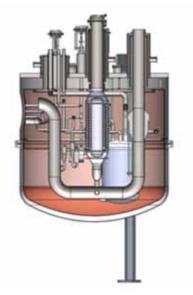
Fig.(5.10)8. Cross section of the distribution box with two heat exchangers.
