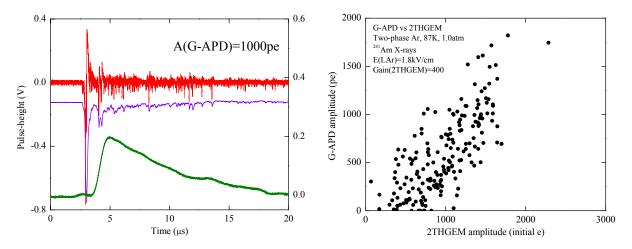
Fig.(1.8)2. Illustration of the Ar operation of the two-phase THGEM-based avalanche detector with optical readout using G-APD at an avalanche gain of 400. Left: a typical scintillation signal (top and middle) and a charge signal (bottom) at a scintillation signal amplitude of 1000 photoelectrons. Right: correlation between the amplitudes of scintillation and charge signals expressed in G-APD photoelectrons and primary (before amplification in the THGEM) electrons.
