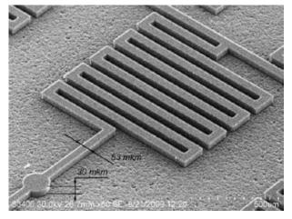
Fig.(6.1)8. Fragment of a work-piece of X-ray mask (an SU-8 structure before the galvanic deposition of gold).
