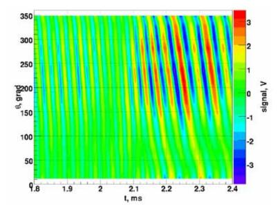
Fig.(4.1)3. The characteristic signal form from azimuthal set of probes (oscillations of the magnetic field radial component). Key stages: 0-1 ms – no large-amplitude oscillations with a distinct frequency; 1-2 ms – oscillations with azimuthal number m = 1; 2.4 ms – oscillations with azimuthal number m = 2; > 4 ms – plasma decay, oscillation frequency decreases significantly over the period of oscillations.
